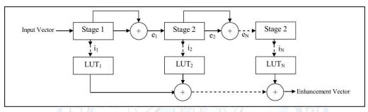
Figure (2): Multistage Vector Quantization System
