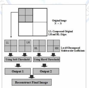
Figure (5): flow diagram of the proposed Multiwavelet thresolding method
