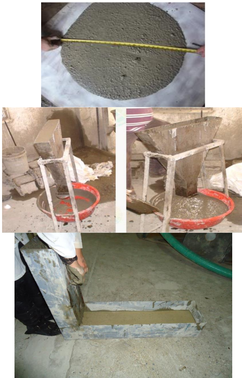
Figure 5. Self-compacting concrete tests (slump flow, V-funnel and L-box)
