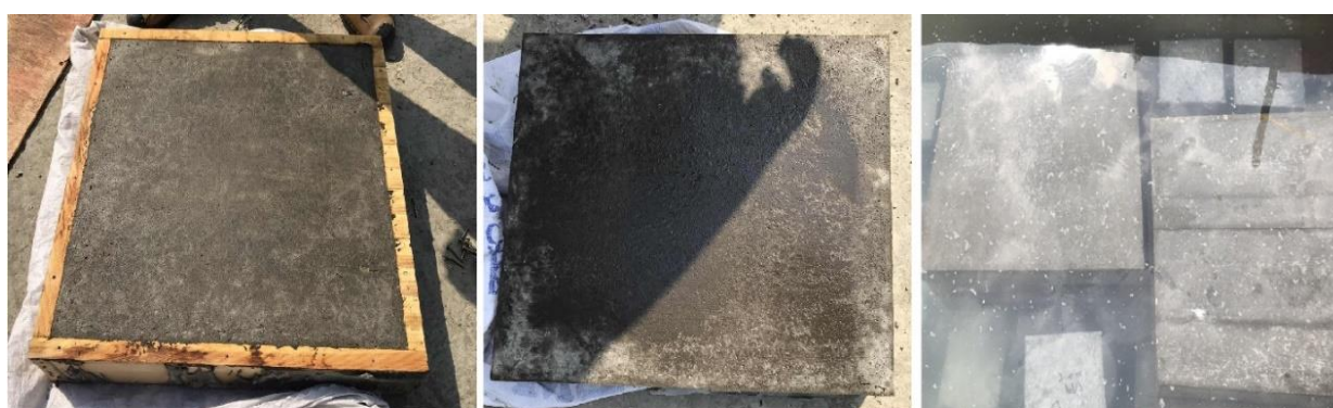
Figure 6. Opening the molds and submerging the slabs in water for curing
