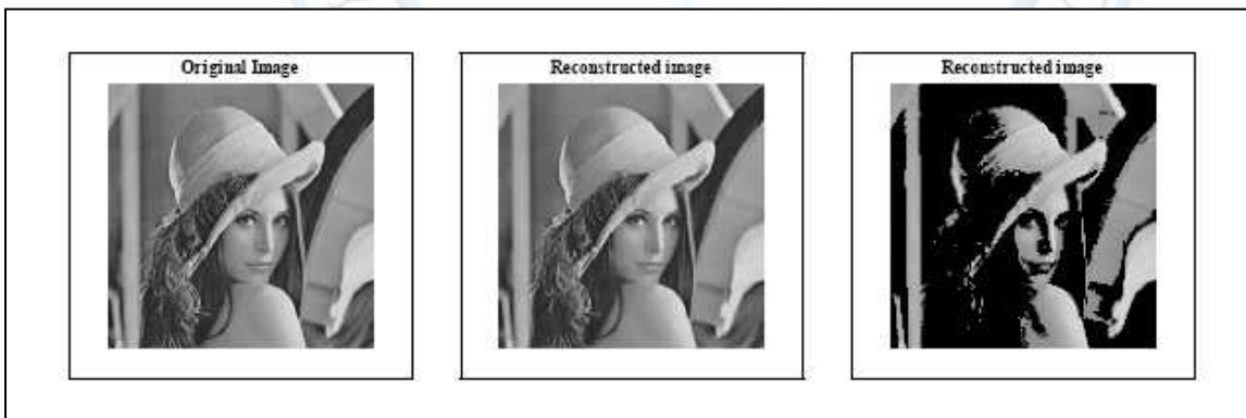
Fig. 5 (a) Original image (b) Reconstructed image using multiwavelet transform (c) Reconstructed image using scalar wavelet
