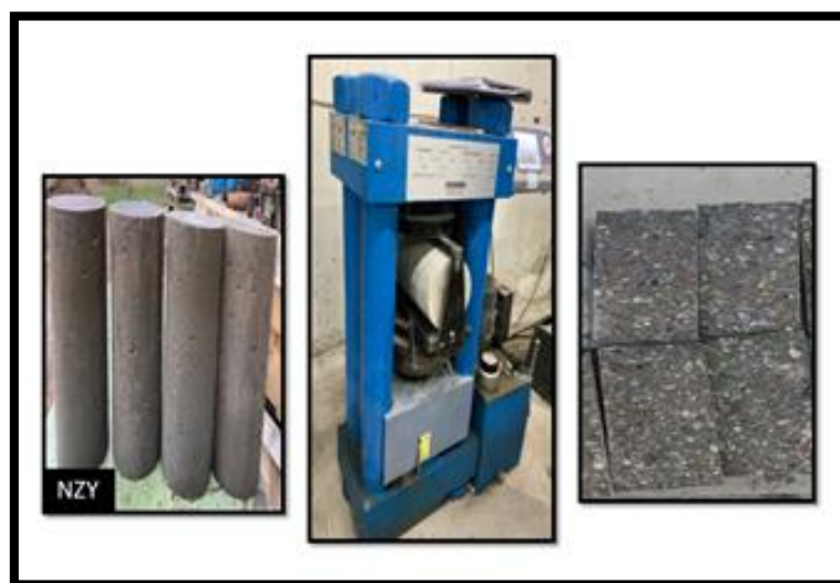
Figure 3. Shows splitting tensile strength test
