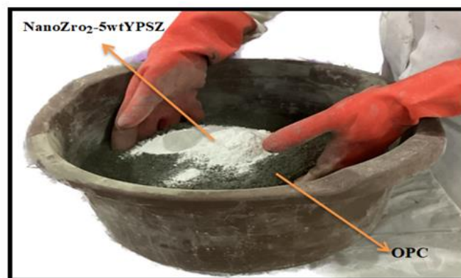
Figure 1. Manual mixing cement with nano zirconia
