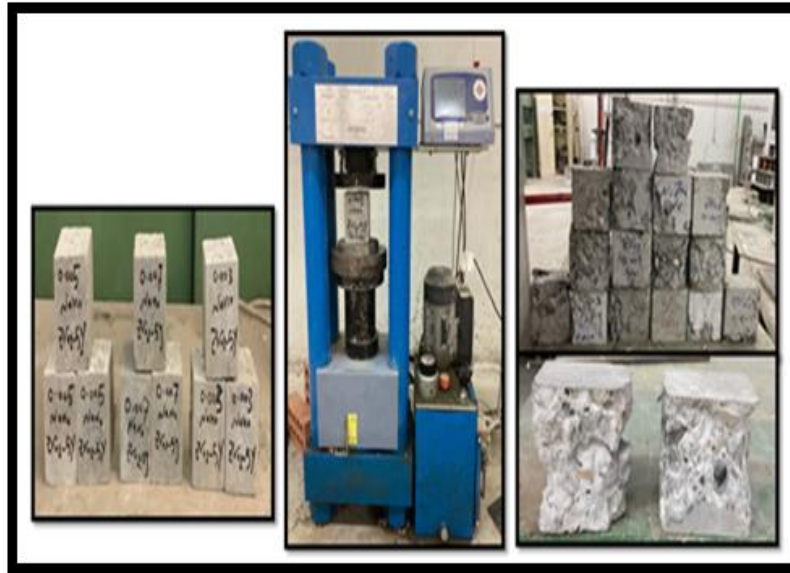
Figure 2. Shows compressive strength test
