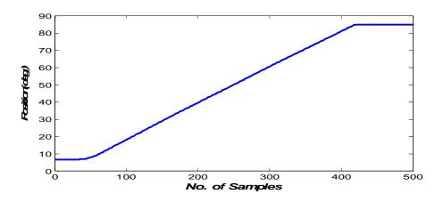
Figure (3) position of the SS exited by a 1-volt step command input
