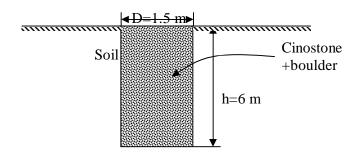
Fig.(2) Dimensions of stone pile body
