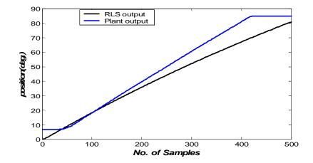
Figure (4) position of the SS exited by a 1-volt step command input and the RLS estimated position exited by the same input.
