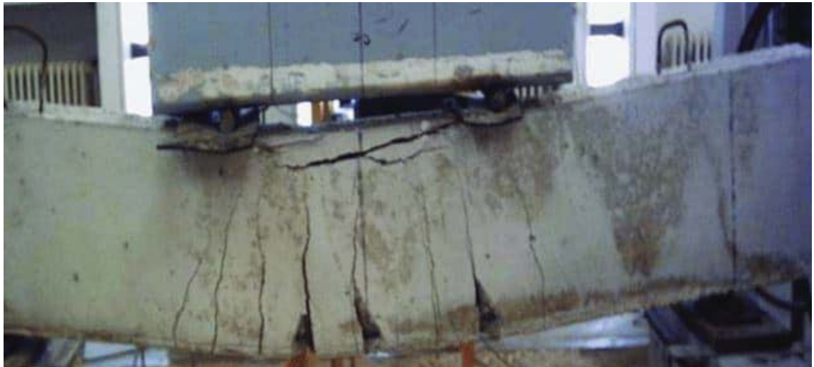
Plate (1-1) Beam Breakage Due to Flexure (Madeh Izat 2020)
