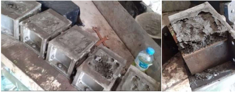
Plate (1-1): The separate and rise up of the foam layer from concrete due to the increased mixing time in the presence of the superplasticizer
