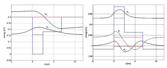
Figure 4: Quantum well structure and wavefunctions without external field
