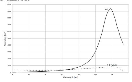
Figure 9: Absorption with and without external field effect
