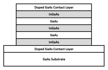
Figure 1: Basic layout of QWIP
