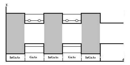
Figure 2: Electronic structure of QWIP
