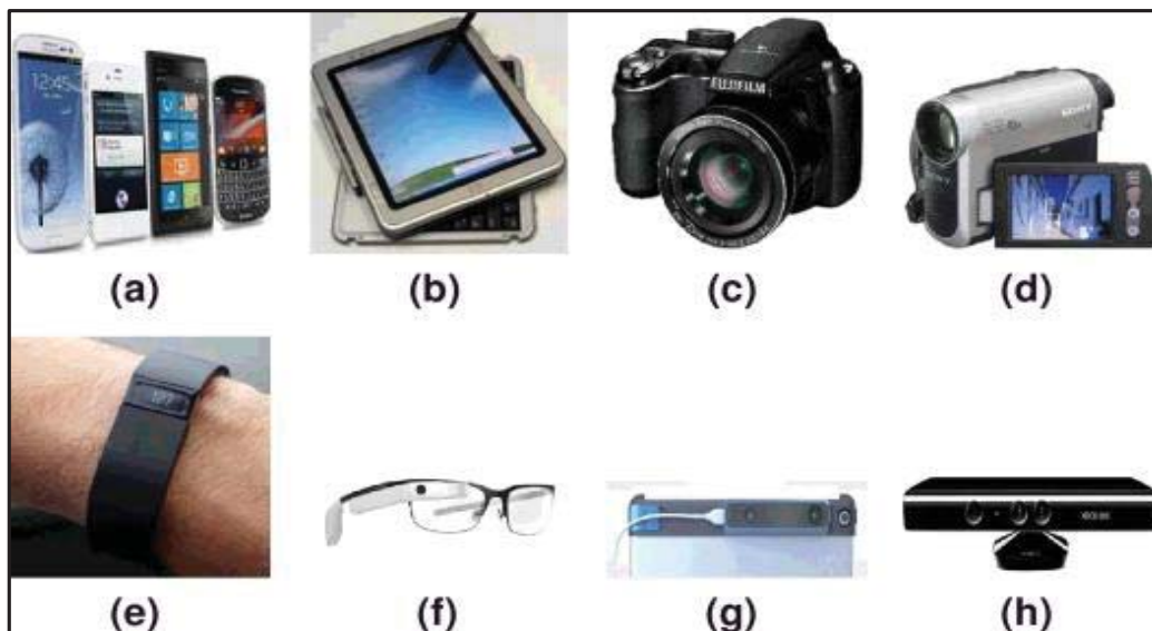
Figure (1.1) : Examples of mobile devices capable of capturing biometric data: (a) smartphones, (b) tablet computers, (c) digital cameras, (d) digital video recorders, (e) wearable activity trackers (e.g., Fitbit), (f) wearable head-mount displays (e.g., Google Glass), (g) 3D sensors [e.g., STRUCTURE (2014)], and (h) portable game consoles (e.g., XBOX Kinect)[1].
