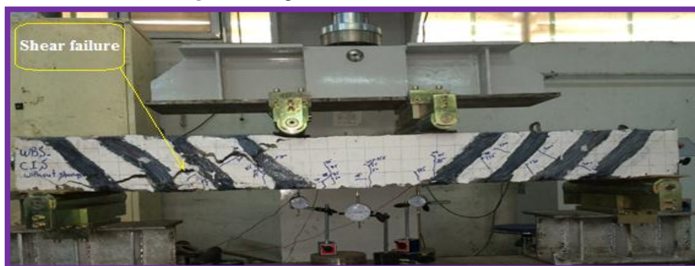
Figure 15: Failure of concrete for (WBS-CIS)
