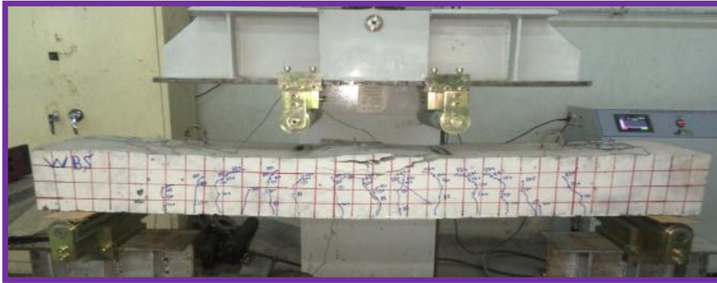
Figure 16: Failure of concrete for (WBS)
