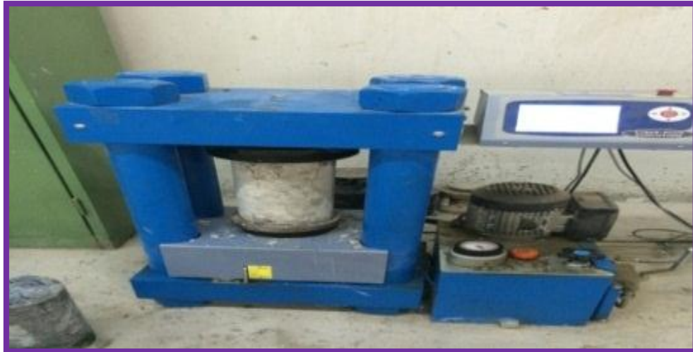
Figure 7 : Concrete Compressive Strength (Cubes and Cylinders)
