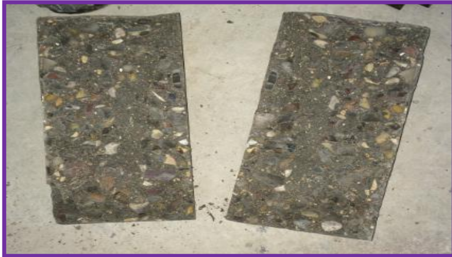
3- Modulus of rupture (prism). According to ASTM-C78 [17]. The test of specimen is shown in Figure 9.
