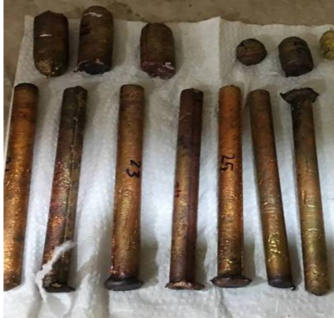
Figure 3: shown the rod casts ingot that produced by stirr casting
