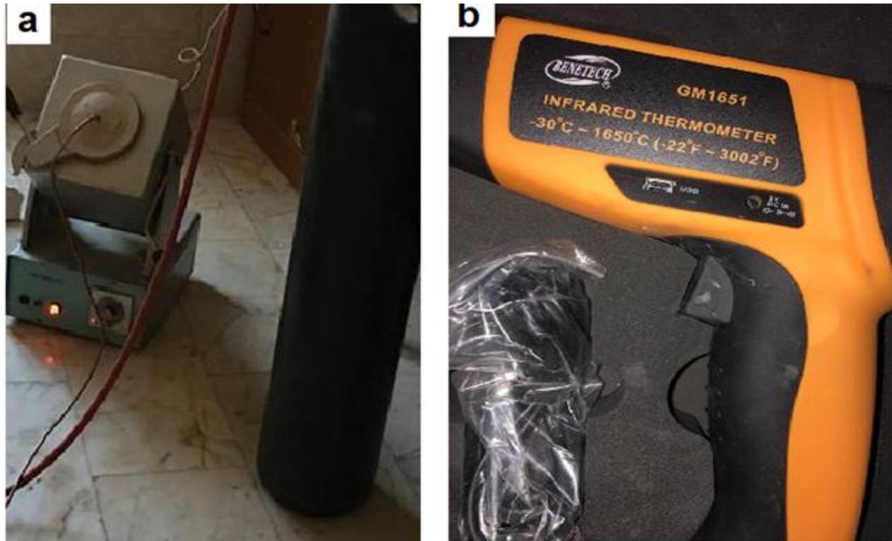
Figure 2: shows (a) solution treatment furnace, (b) Thermometer infrared.
