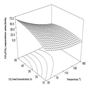
**Figure 6:** Effect of temperature and CO<sub>2</sub> feed concentration on CO<sub>2</sub>/CH<sub>4</sub> separation selectivity at pressure difference across the HT-silica membrane of 300 kPa
