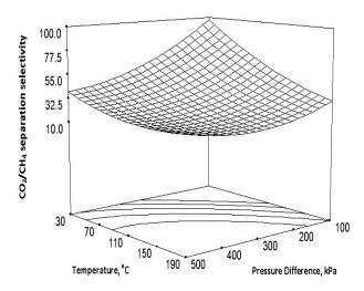
**Figure 4:** Effect of pressure difference across the HT-silica membrane and temperature on CO<sub>2</sub>/CH<sub>4</sub> separation selectivity at 30% CO<sub>2</sub> feed concentration
