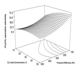
**Figure 5:** Effect of pressure difference across the HT silica membrane and CO<sub>2</sub> feed concentration on CO<sub>2</sub>/CH<sub>4</sub> separation selectivity at temperature of 110 °C
