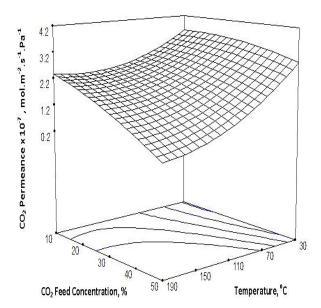
**Figure 3:** Effect of temperature and CO<sub>2</sub> feed concentration on CO<sub>2</sub> permeance at pressure difference across the HT-silica membrane of 300 kP<sub>2</sub>
