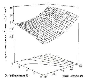
**Figure 2:** Effect of pressure difference across the HT-silica membrane and CO<sub>2</sub> feed concentration on CO<sub>2</sub> permeance at temperature of 110 °C
