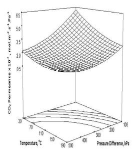
**Figure 1:** Effect of pressure difference across the HT-silica membrane and temperature on CO<sub>2</sub> permeance at 30% CO<sub>2</sub> feed concentration
