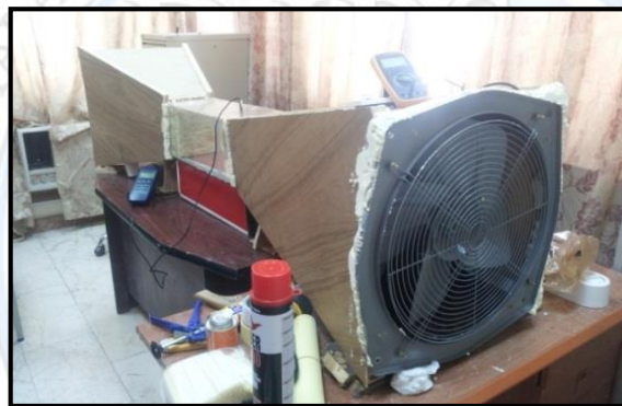
Figure (5) The fabricated design of wind tunnel
