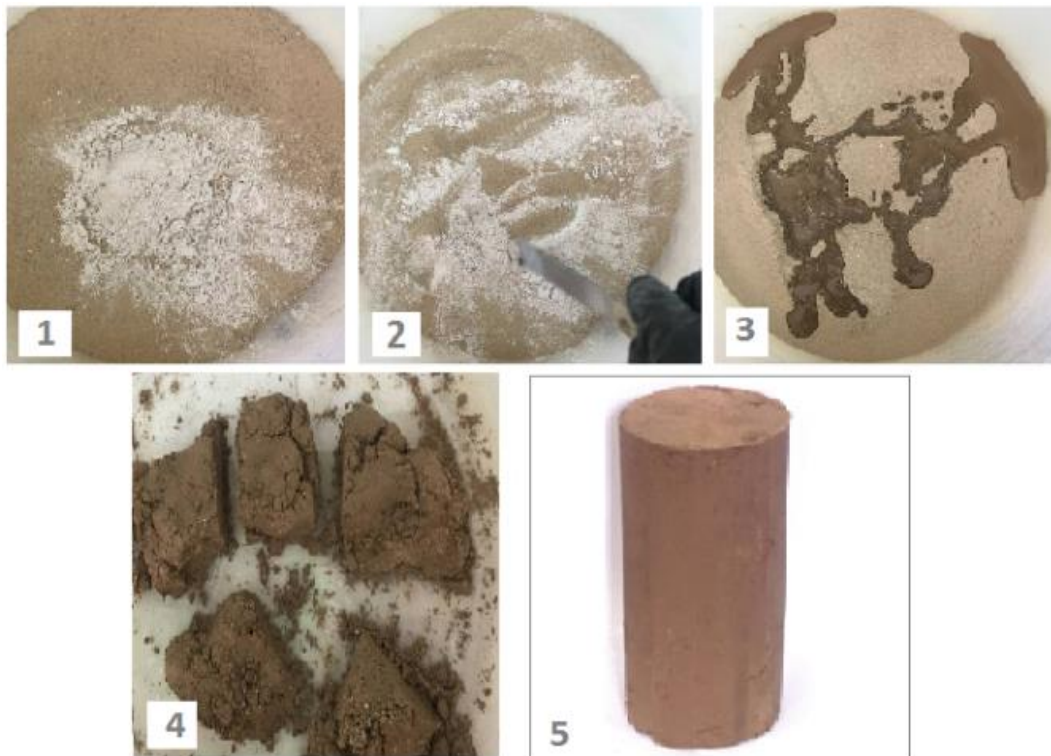
Figure. 1 Steps of mixing Metakaolin-soil with activator
