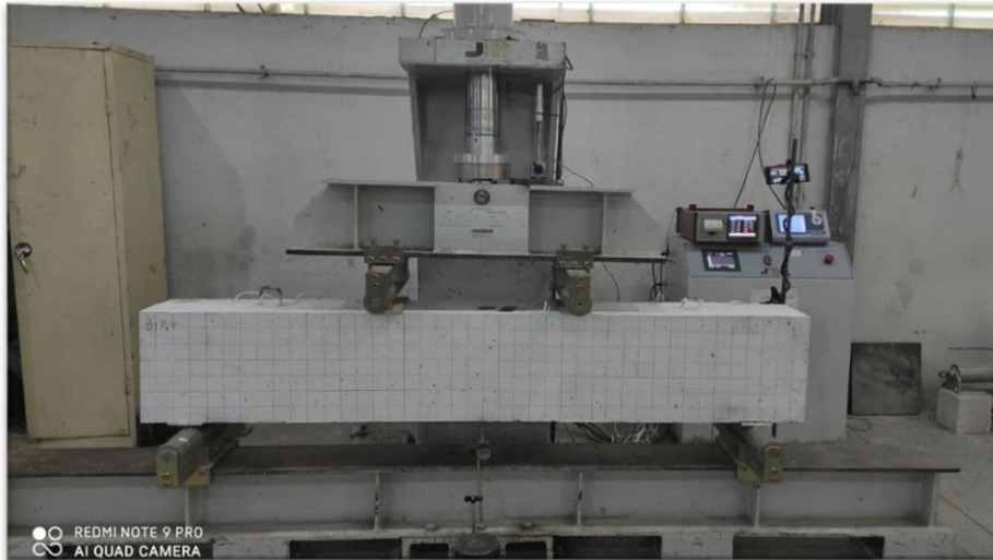
Figure 3. Position of beams in the load-testing machine
