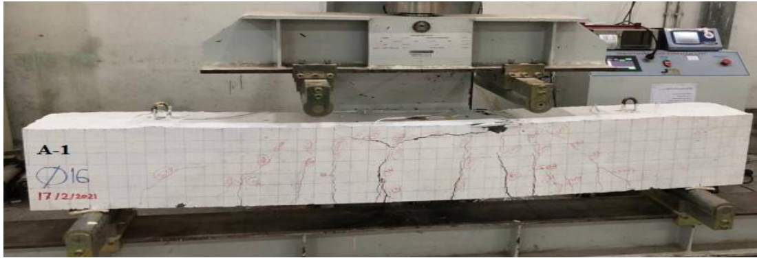
Figure 5. Crack pattern of A-1
