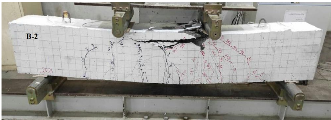
Figure 7. Crack pattern of B-2.
