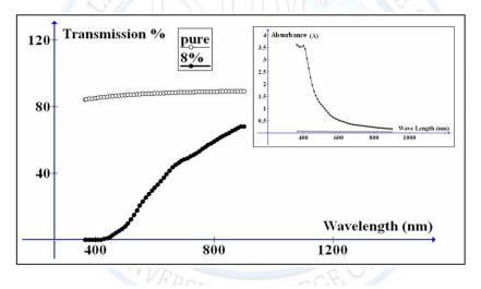
Figure (1) Transmittance against Wavelength for pure PVA , 8wt% KMnO4 doped PVA samples. The inset shows the Absorbance vs. Wavelength.
