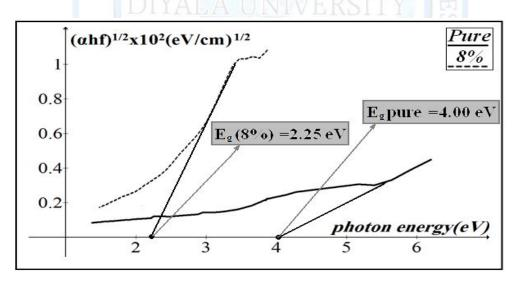
Fig. (3) Optical energy band gap of pure PVA , 8 wt%, KMnO<sub>4</sub> doped PVA samples.
