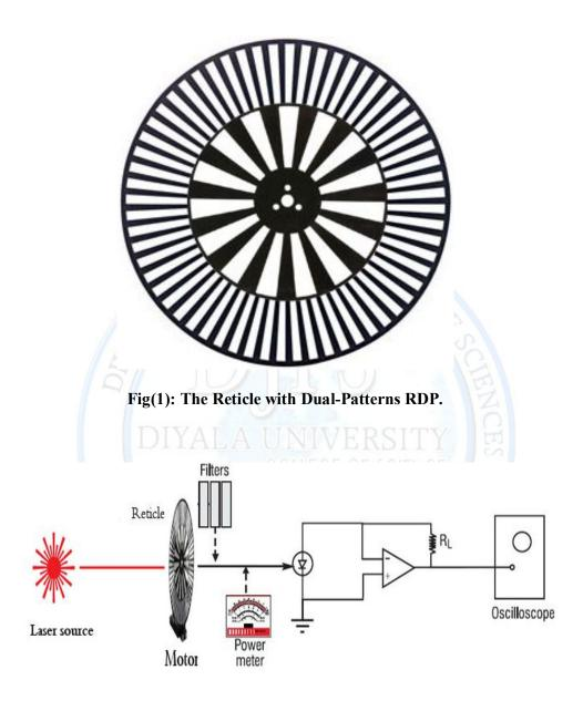
Fig (2): The location of reticle in the optical system
