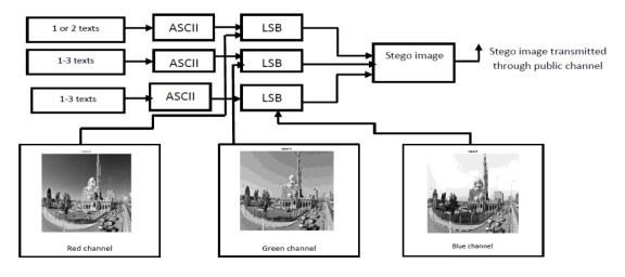
Figure (2) Embedded System for Text.
